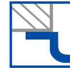
Countertop edge sits back from the edge of the sink, exposing the sink rim, typical 1/8".
