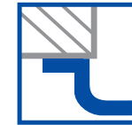
Countertop extends over the edge of the sink.
